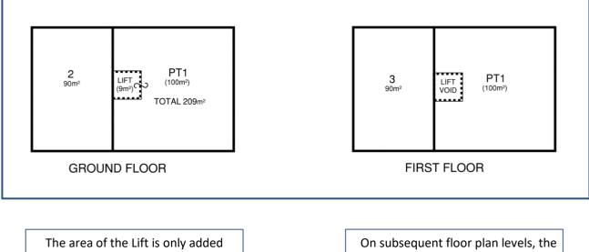
once to the overall area of the lot. In this example it is added to the ground floor level On subsequent floor plan levels, the Lift Void is shown as above.
